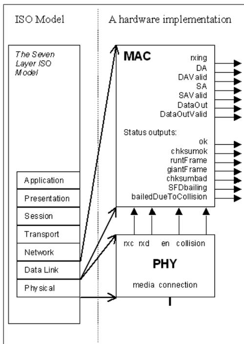
The diagram shows the ISO seven layer reference model on the left. On the right is a block diagram of the hardware for the two layers which are of concern for this design.
