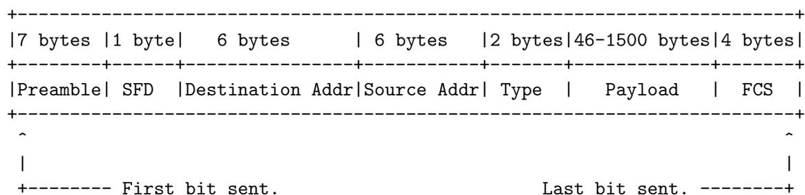
SFD is Start of Frame Delimiter. It is the bit pattern 10101011. The very next bit after the SFD is the first bit of the Destination Address (DA).
